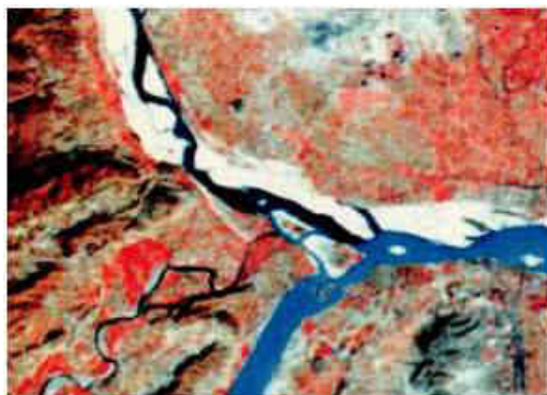
Fig.7: Hyperspectral image of the confluence of a river (black) and a polluting stream (Blue). Artificial colors adjusted on the basis of scattered of sunlight from different regions. Clean water of river reflects much less than the suspended particles in the polluted water, whereas reflection from white sand is the largest [Courtesy Prof. K N P Raju, Geography Dept., BHU]
